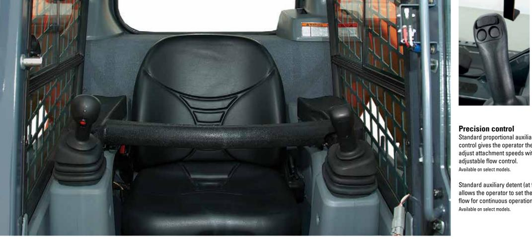
Standard proportional auxiliary hydraulic control gives the operator the ability to adjust attachment speeds with infinitely
